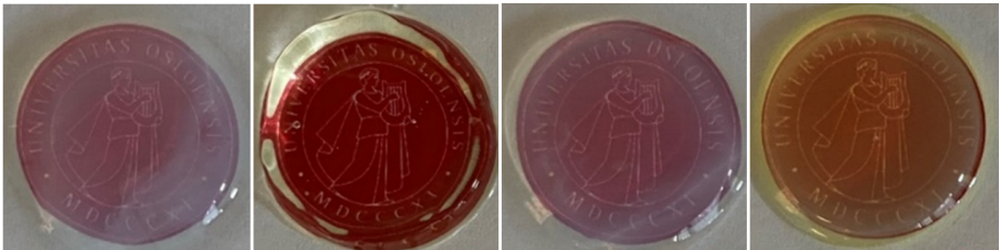
Figure 4.2: Photographs of collagen hydrogel formulations, illustrating the difference in optical properties. From left to right: Col gel, LC gel, CD gel and RF gel.
