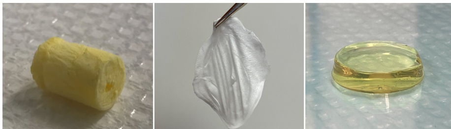
Figure 4.1: Photographs of collagen formulations prepared in Paper I-IV . From left to right: RF photocrosslinked collagen sponges, collagen-NADES sheets and LC photocrosslinked collagen hydrogels.
