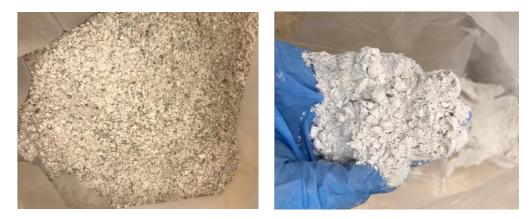
Figure 4. Grinding oyster shell to create aggregate (0-4 mm) and powder (150 µm).
