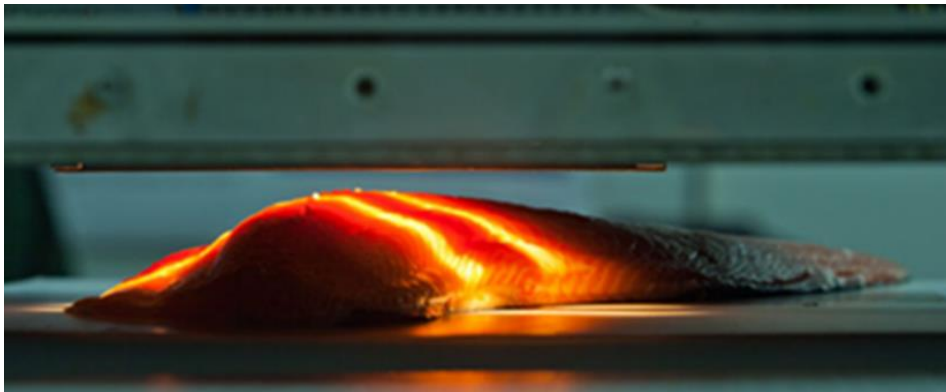
Photo 1 Instrumental reading of a rainbow trout fillet at a rate of 50 cm per second
