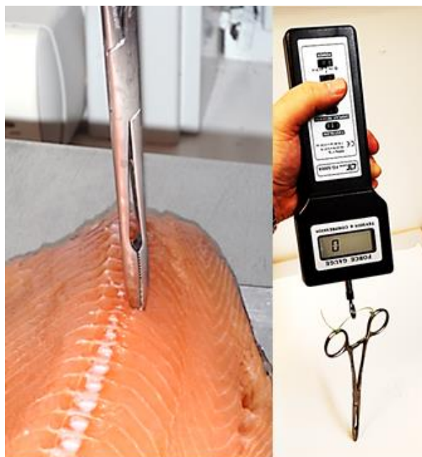
Photo 2 The photo on the left shows a clip being attached to the end of a pin bone in a salmon fillet. The photo on the right shows the actual measurement set up.
