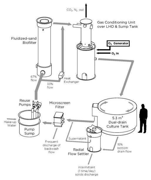
Fig. 1. Water flow and process design for an individual recirculation aquaculture system.
