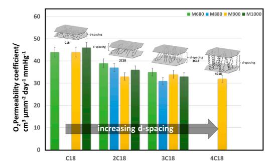
**Figure 6.** Effect of clay organic modifier on the macroscopic properties of polymer nanocomposites (PNCs). Montmorillonite with CEC/ $\mu$ eq g<sup>-1</sup> of 680, 880, 900, and 1000 were chemically modified with trimethyl-(octadecyl)ammonium (C18), dimethyldi(octadecyl)ammonium (2C18), methyl-tri(octadecyl)ammonium (3C18), and tetra(octadecyl)ammonium (4C18) and dispersed within a linear high-density poly(ethylene) (HDPE) matrix [1,55].
