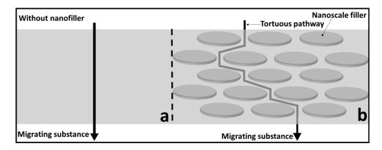
**Figure 4.** Schematic of the gas molecule diffusion through (**a**) a polymer-only barrier and (**b**) a polymer composite barrier. Uniformly dispersed nanoplates decrease the permeability by increasing the resistance through tortuosity. Adapted from [1,7].
