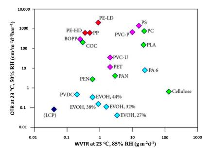
**Figure 2.** Oxygen permeability (OP) and water vapor transmission rate (WVTR) normalized to a thickness of 100 μm for different polymers. Source: Fraunhofer IVV [7,23].
