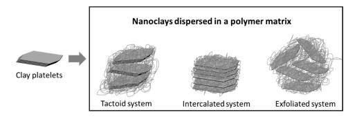
Figure 5. Tactoid, intercalated, and exfoliated polymer-clay systems. Adapted from [52].
