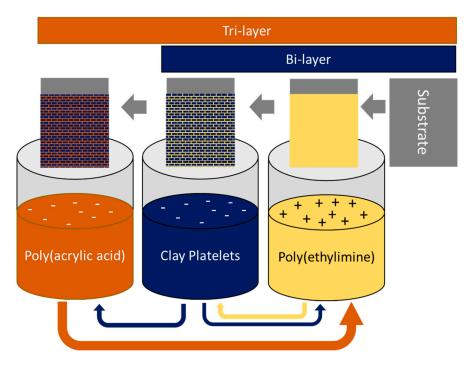
**Figure 7.** Layer-by-layer deposition process for bi- and tri-layer systems with the alternate adsorption of charged polymer and nanoclay platelets. Adapted from [99].
