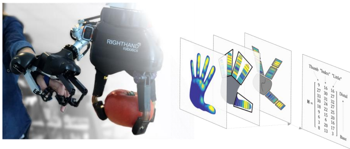
Figure 2. Mapping human interactions with objects to establish an understanding of sensor importance during handling actions. This enables a better understanding of contact importance for an AI., creating a key that can be used to weight sensor input when grasping is AI-controlled.
