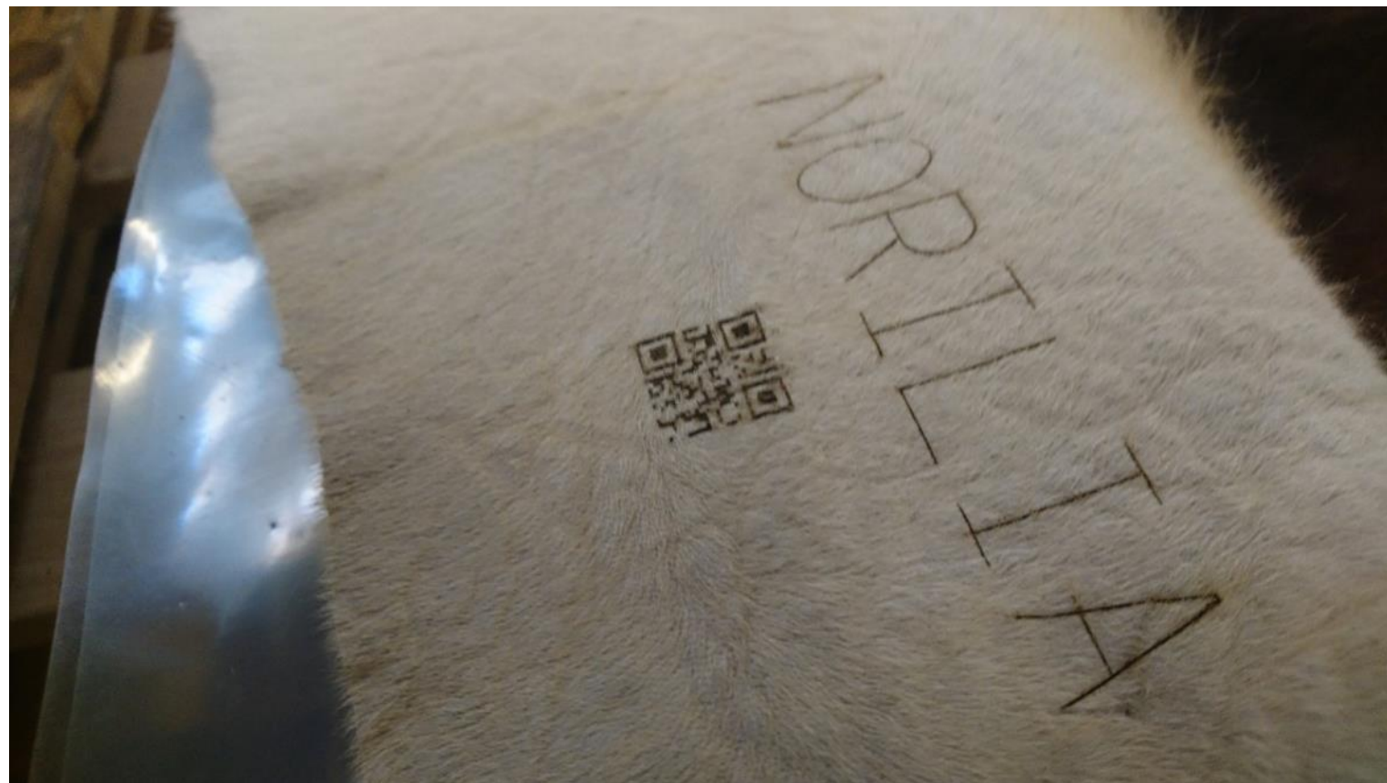
Figure 2. An example of a laser-tagged hide taken from tests carried out in collaboration with Norilia.
