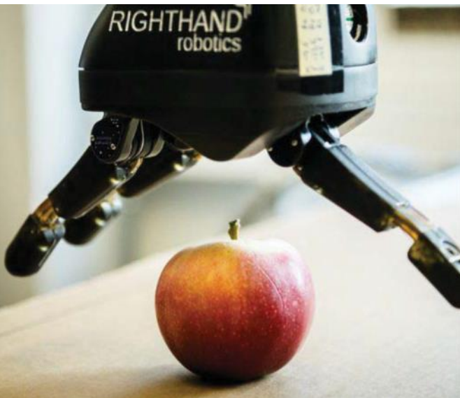
Figure 1. The robotic handling of food items using current technology. A gripper mounted with sensors along each finger that sense interaction forces and facilitate gentler touch.
