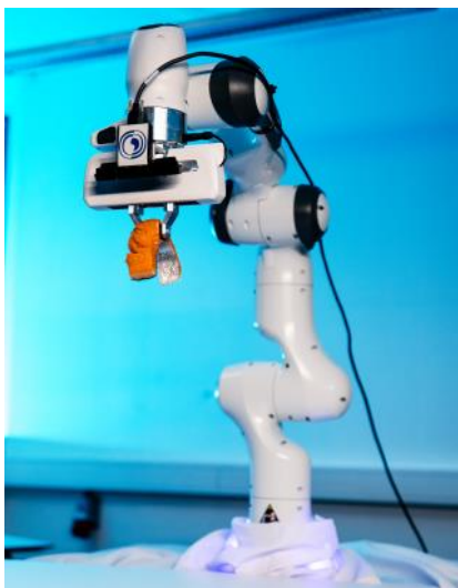
Figure 1. Grasping of a salmon filet portion. The VS-assisted grasping agent was not presented with any instances of the salmon during training in simulation or the real world, demonstrating that the agent generalizes well to previously unseen objects.
