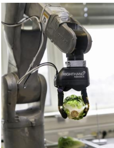
Figure 1. Close-up image of an autonomous robot grasping a lettuce based on application of our multi-modal (visual-tactile) robot LfD learning policy.
