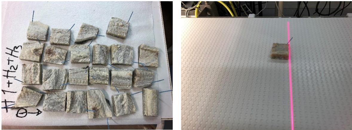
Figure 4 Labelled samples prepared for 3D imaging (left) and 3D imaging on a conveyor belt (right) (Photos: G. Lorentzen, Nofima).
