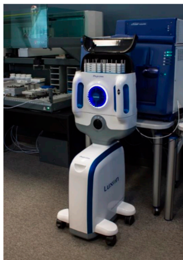
Figure 3. Laser diode thermal desorption ion source tandem mass spectrometry (LDTD-MS/MS) analysis (Source: [61]).
