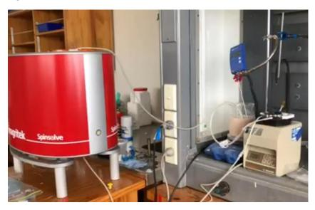
Figure 1: Image of the online NMR setup for monitoring of enzymatic hydrolysis
