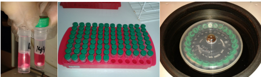
Figure 2: Left-tubes with separated phases, middle – preparation of tubes for tissue homogenization, right – 24 tubes in refrigerated centrifuge.
