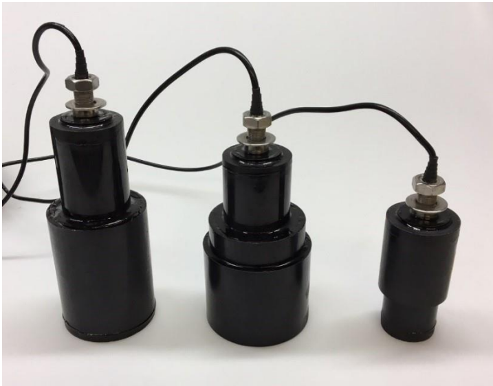
Figure 3: Ultrasound transducers used in the experiments. From left: BII-7509 (9,3 kHz), BII-7502 (21 kHz), BII-7506 (54 kHz).
