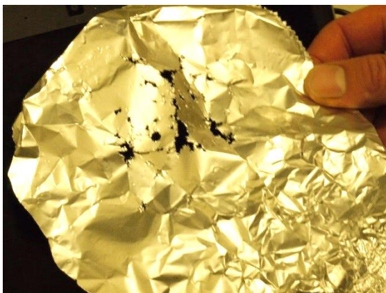
Figure 6: Aluminium foil perforated by ultrasonic cavitation effects.
