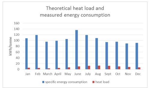
**Figure 7.** Comparing theoretical heat load and total measured energy consumption. Notice that these are for comparison of the magnitudes only, since the energy consumption for removing the heat load is not calculated.
