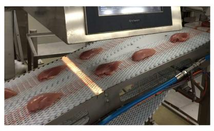
Fig 1. NIR system installed in production line. Illuminating line crosses the entire conveyor belt. All passing fillets were measured.
