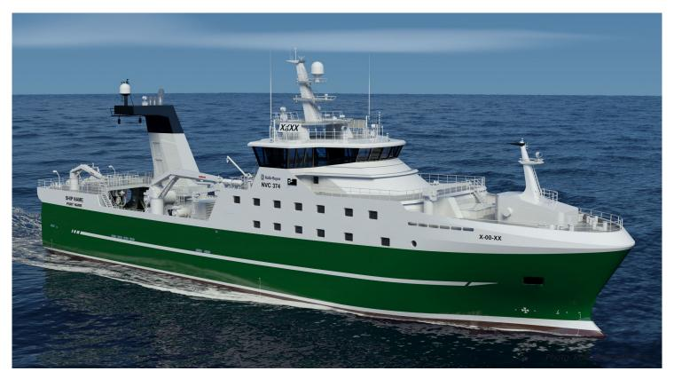
Future trawler with live storage on board may be based on a standard hull 80 meters long and 17 meters wide. Photo: Rolls-Royce Marine.
