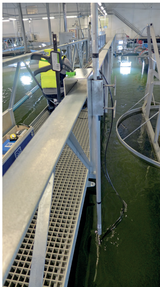
Fig. 4.10. Measuring water velocity in large land-based tanks, in the HYDRO project
