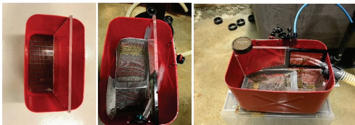
Figure 2 The Spillbox. Water from the outlet passes through the wires on the frame. Aided by the angle of the outlet tube, the pellets bump into the container on the left. The faeces stick to the wires on the frame and is blown into the container below by compressed air.
