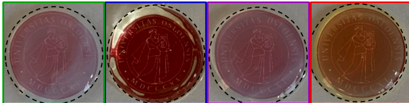
Fig. 2. Appearance of the hydrogels depending on crosslinking procedure. From left: Col gel with translucent appearance, LC gel with slightly yellow and transparent appearance, CD gel with translucent appearance, and RF gel with yellow and translucent appearance. Gel edges are highlighted using dashed lines and the transparency is illustrated by a red logo in the background. (For interpretation of the references to color in this figure legend, the reader is referred to the web version of this article.)
