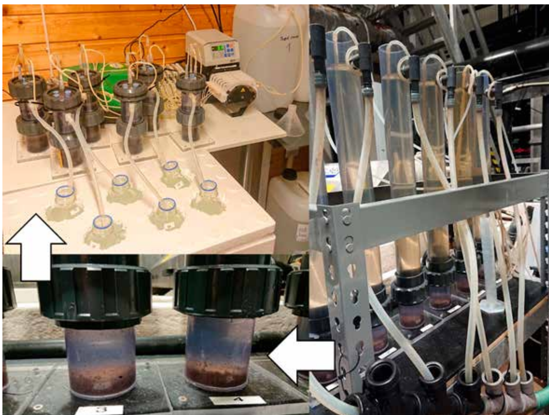
Sediment collection in RAS with up flow columns and testing RAS sediments in flow cells for H 2 S production. Arrows indicate the workflow from sediment collection to analysis. Photo: Andre Meriac, Nofima.
