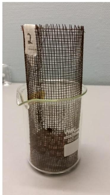
Figure 1 Feed sample in a mesh wire container placed in a beaker for water stability test.
