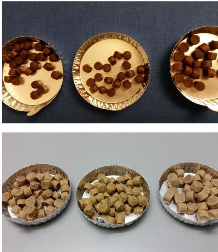
*Figure 4 Experimental feeds eight months after production. Upper panel, from left: Diet 1, 2 and 3. The visual appearance resembled that right after production. Lower panel, from left: Diet 1, 2 and 3 after two hours shaking in water bath in the water stability test. Diet 1 had intact pellets, pellets of Diet 2 had some rounded edges, and Diet 3 had swollen pellets. The difference in visual appearance among the feeds after the water stability test was larger shortly after production.*
