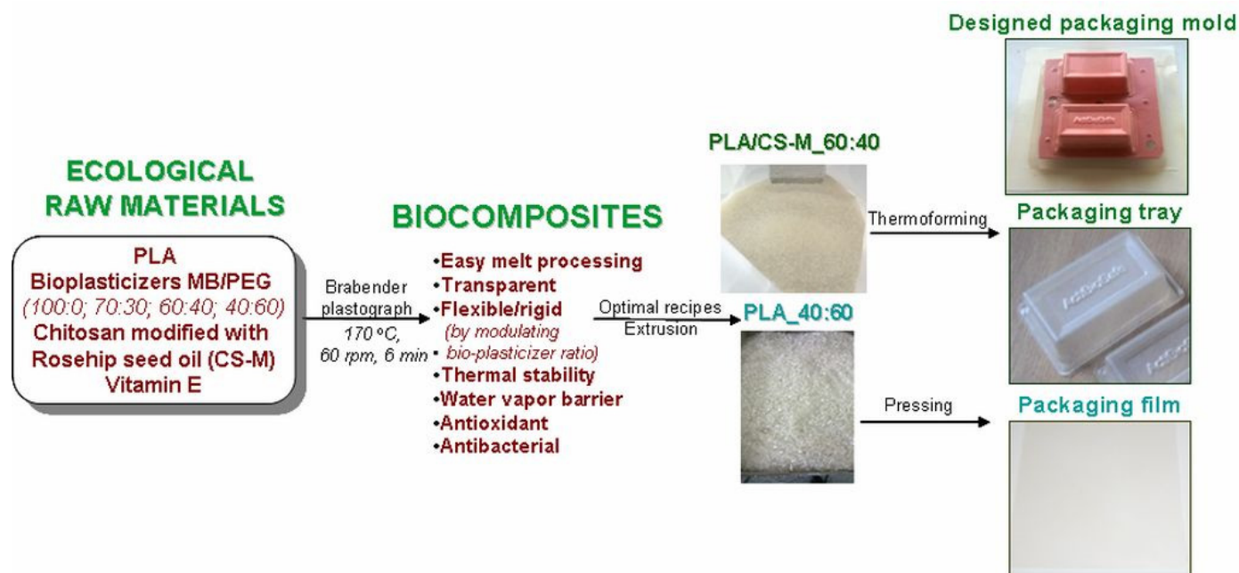
Figure 7. Overview of the main technological steps for obtaining of food packaging system.
