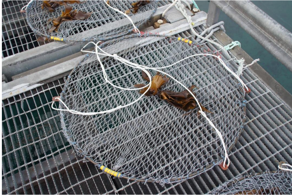
Figure 3 The round collapsible trap (Round trap) tested in the Experimental trap trials (this trap has a single bait station using algae).
