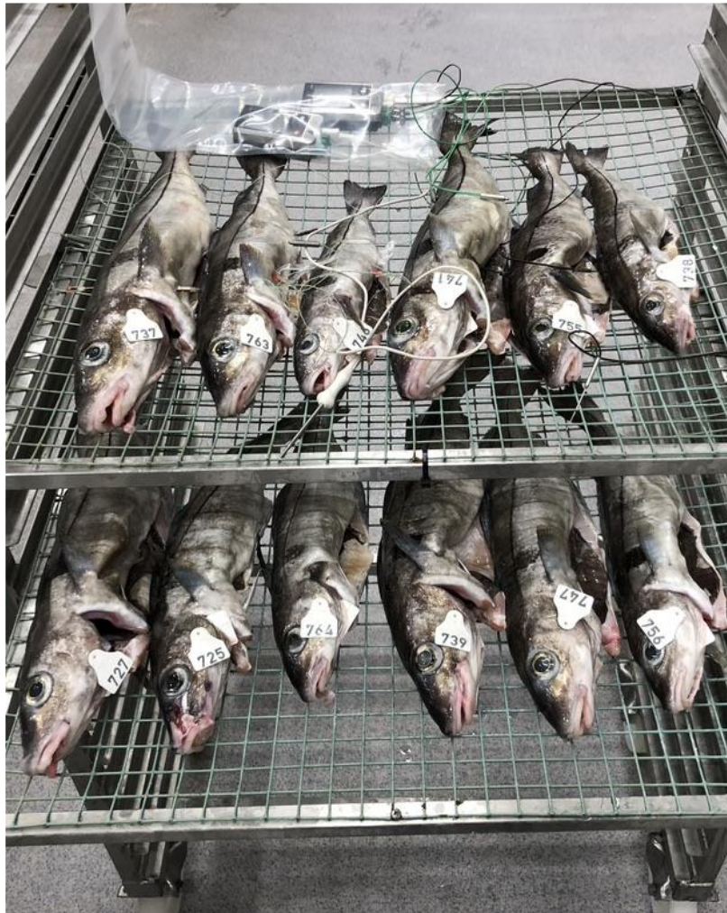
Figur 1 Illustrerer oppsett for tunnelfrysing.
