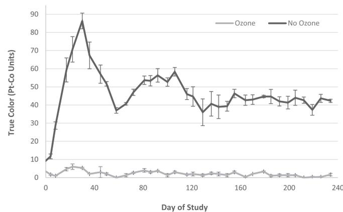
**Fig. 4.** True color (mean  $\pm$  standard error;  $N = 3$ ) in RAS with and without ozone over the study duration.
