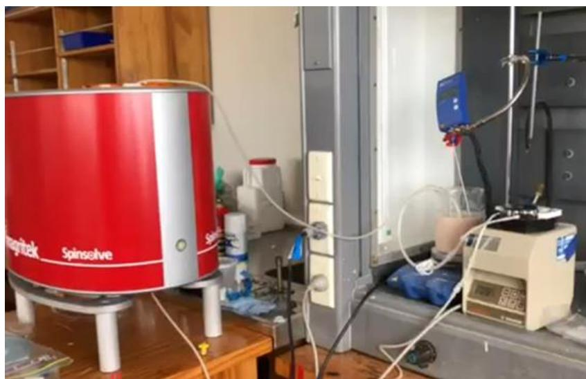
Figure 1: Image of the online NMR setup for monitoring of enzymatic hydrolysis
