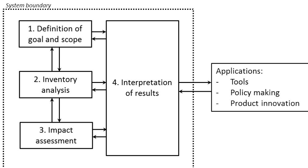
Figure 3 LCA Framework
