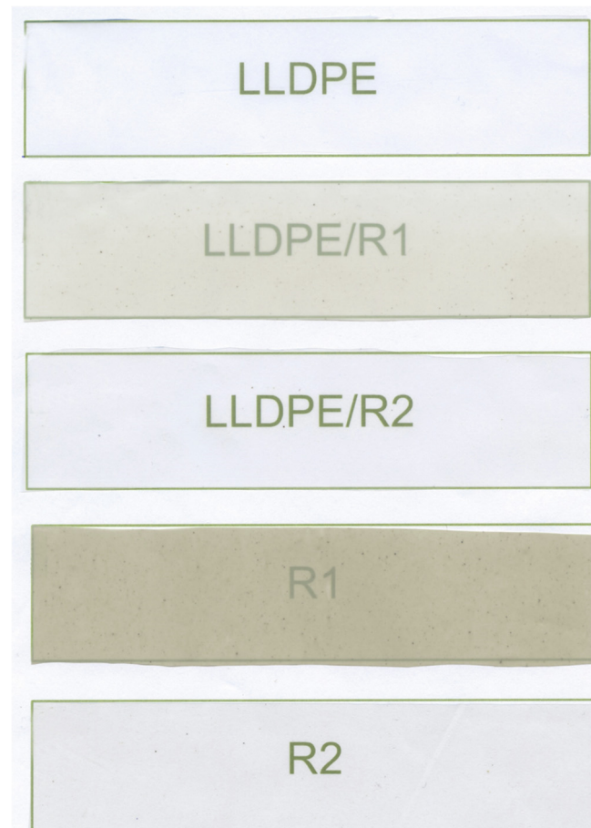
Fig. 6b. 3-layered film samples: LLDPE, LLDPE/R1, LLDPE/R2, R1 and R2.
