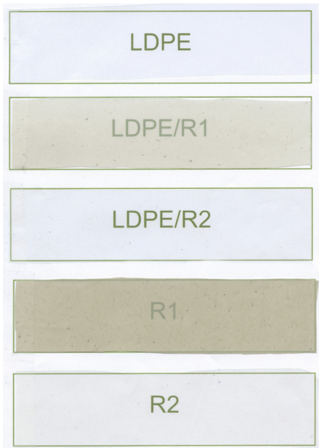
Fig. 6a. 3-layered film samples: LDPE, LDPE/R1, LDPE/R2, R1 and R2.
