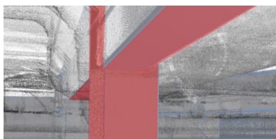
Fig. 5. Comparing fit with existing 3D building model with point cloud.
