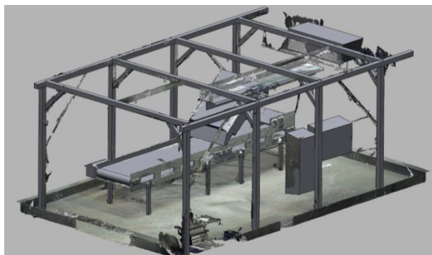
Fig. 2. Hybrid model of point cloud and solid models.
