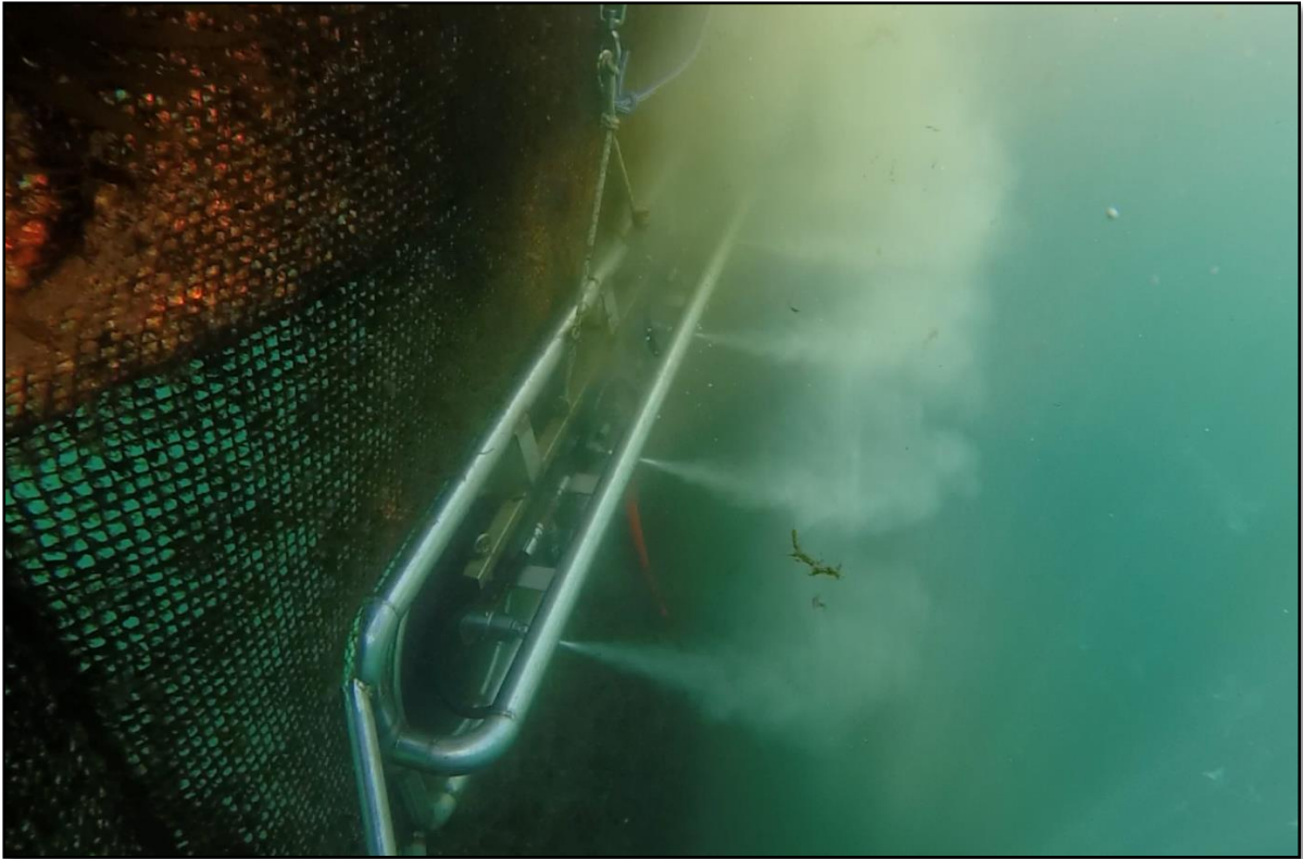
Figure 2.2.4-2. Example of a net cleaning rig from AKVA in action on a net with relatively low levels of fouling. Photograph courtesy of N. Ribeiro, with permission.
