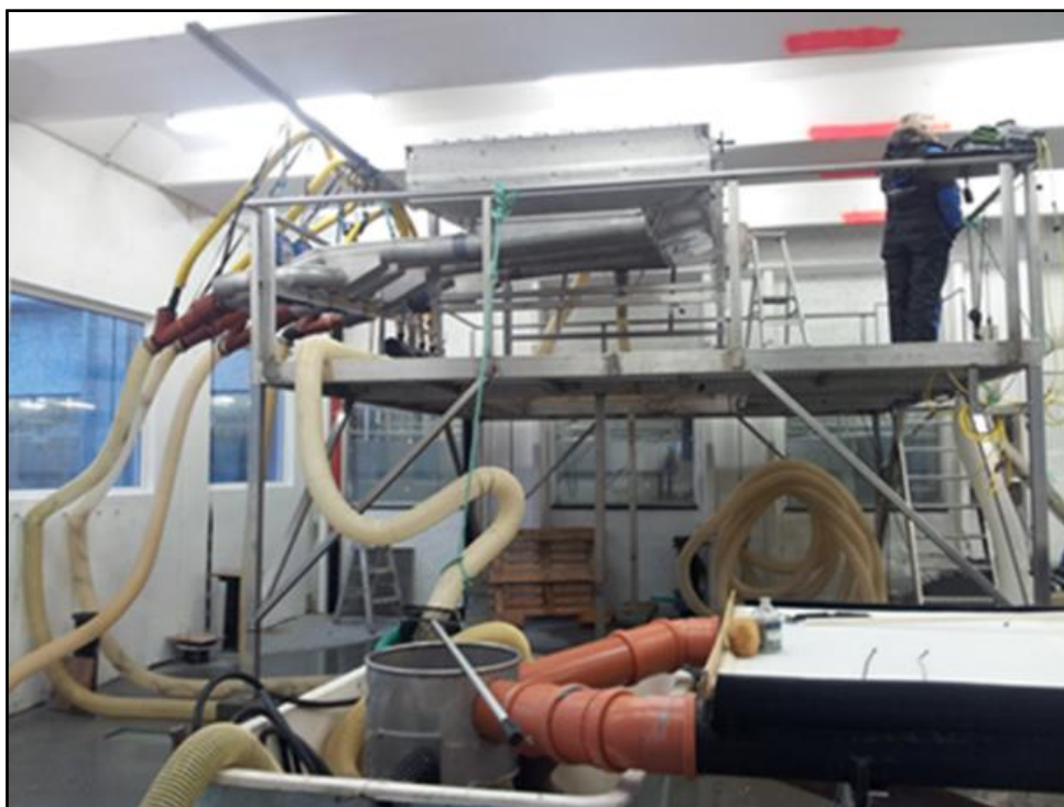
Figure 1.2-1. Pipe bends may cause damage to the fish. Photo: Å. M. Espmark
