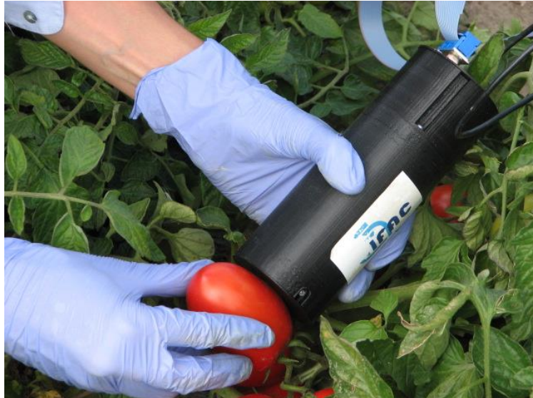
Figure 4 In-field tomato lycopene monitoring by use of a LED fluorescence sensor
