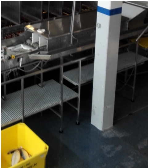
Fig. 1. Some of the challenges in a salmon processing plant. Notice the different height levels between the floor and the walkway, the narrowness of the walkway and the cables hanging from the roof down to the machine.
