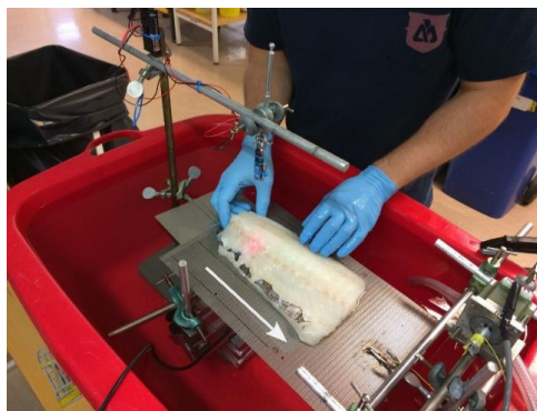
Figure 3. Complete setup placed in a plastic tub for immersion in water. The fish fillet is placed on a perforated plate with a slit in the middle to allow the ultrasound to pass through to the fillet. The plate is pulled by a stepper motor in the direction of the white arrow. A laser pointer mounted above the fillet indicates the position of the transducer focal point, enabling the operator to aim the ultrasound at the bone row during continuous treatment.
