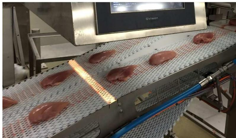
**Fig 1. NIR system installed in production line.** Illuminating line crosses the entire conveyor belt. All passing fillets were measured.
