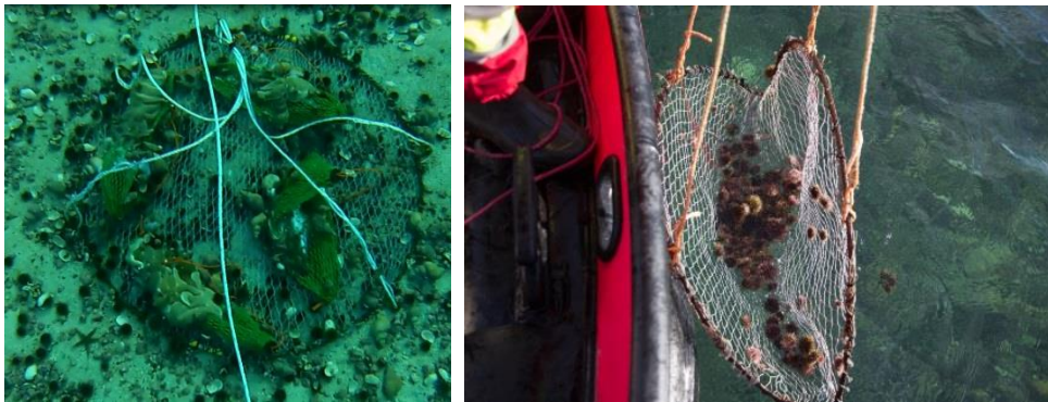
Figure 12 The round collapsible traps designed and tested by Nofima in Norway; sitting on the bottom (left) and being pulled into the boat (right).
