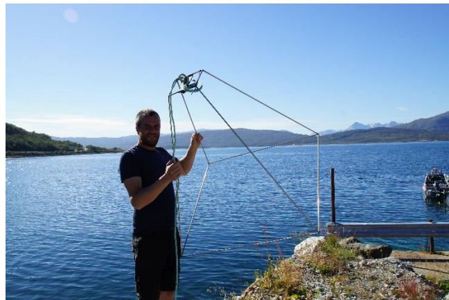
Figure 9 The steel frame used for fixed frame camera surveys in Norway.
