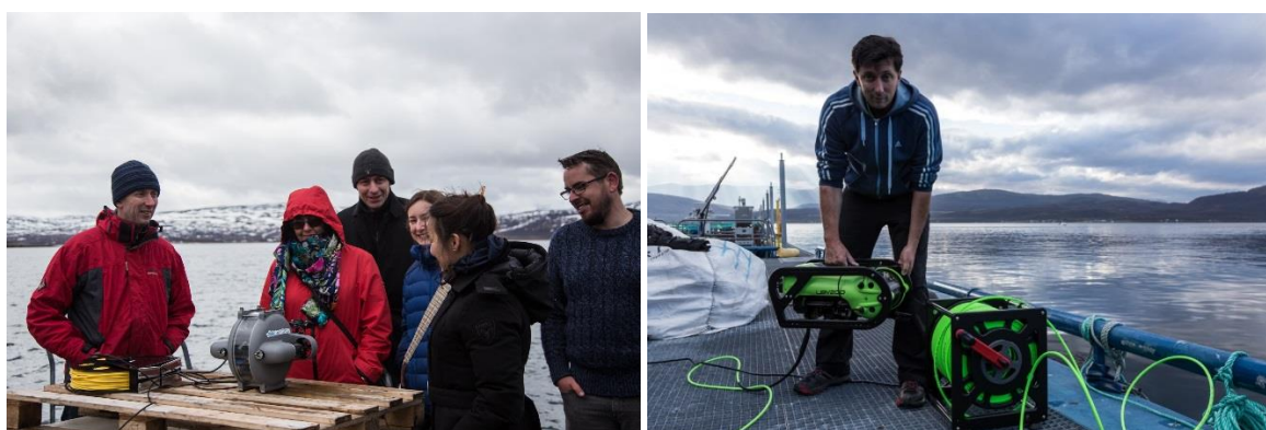
Figure 8 The mini ROVs tested by Nofima in Norway for rapid initial site surveying for urchin abundance; Left) the deep trekker, Right) the SeaBotix LBV300-6 mini ROV.
