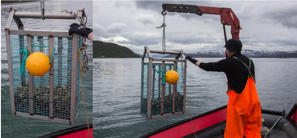
Figure 6 The mini-dredge used in the Nofima trial, left and the dredge being pulled onboard (right).
