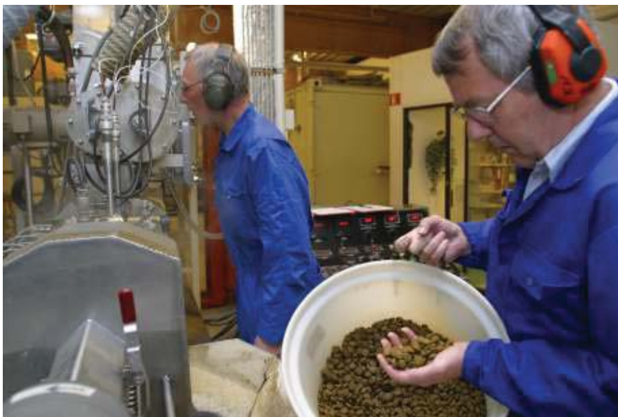
Figure 4 Experimental production of dry feed pellets for sea urchins.
